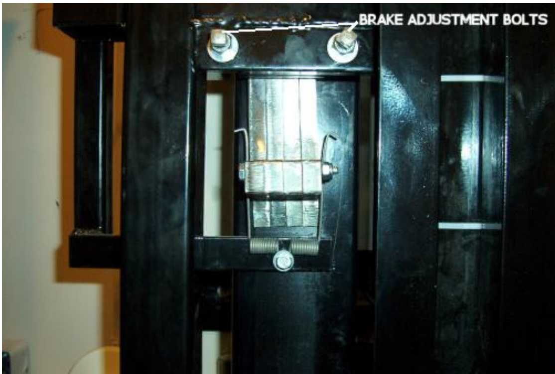
Figure 2. Location of brake adjustment bolts.
